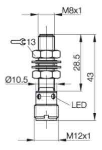
Inductive Sensors BES M08EE-NSC15B-S04G M8x1 x 43 normally-open Sn=1,5mm shielded
